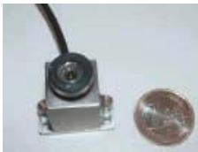
MR compatible black & white camera with f=2.5mm and f=6mm lenses on a ball-joint. Used to monitor volunteer in the bore and can be used for recording subject hand movements, etc.
