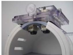
The SV-7021 is a binocular visual system designed for MR use. The 7021 system accepts dual, independent XGA inputs (1024x768). The SV-7021 system can be combined with the eye monitoring system to enable simultaneous visual presentation and eye tracking for one or two eyes.
