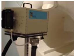
The SV-6011 is a color LCD projection system designed for MR use. The 6011 system accepts an XGA input (1024x768). The projector displays images on a rear projection screen that hangs in the bore.
